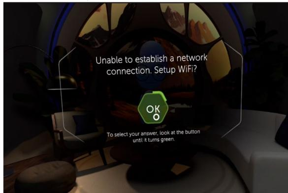
To make selections, the operator moves their head to direct the pointer and holds the pointer over the desired target until selected.
