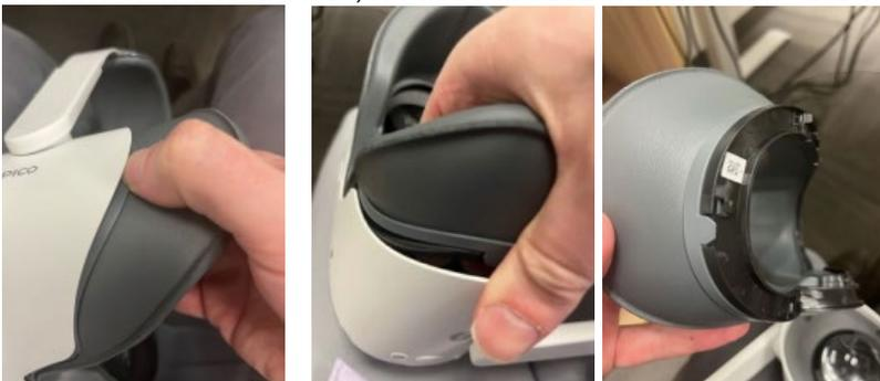
Gently separate the black insert from the old facemask and attach it to the new facemask and ensure the mating point clips in properly.
